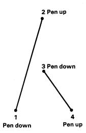
The digitized coordinates and pen status information are stored in the numeric arrays  $X \subseteq I$ ,  $Y \subseteq I$ , and  $P \subseteq I$ . To reproduce the digitized image, enter the following multi-statement line and press  $\overline{\text{END LINE}}$ . Be sure your plotter is equipped with paper and a pen.
