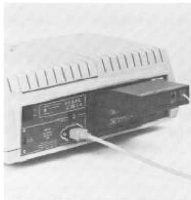
Figure 1-4. Modem Installation Photo
