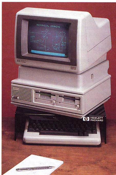
Use these convenience accessories to: (1) tilt display up/down and (2) swivel equipment right/left for easiest use, and (3) park keyboard out of the way when not in use.
