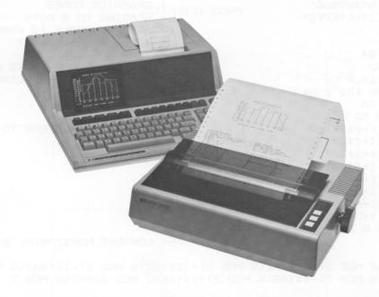
Hardcopy images of CRT graphics can be generated using the BASIC programs listed below. Binary utility routines also exist for this purpose and are available through the HP Series 80 Users' Library. These utilities will provide a single-command copy capability and will copy much faster than the BASIC routines. Ordering information for these is given at the end of this note.
